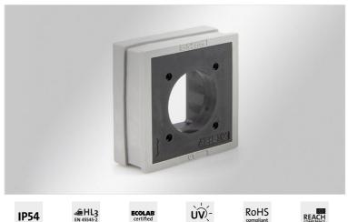
The grommet QT-AT-FL is constructed on the basis of a large QT cable grommet. The polyamide body is moulded with elastomer. All square flanges with dimensions  $19.8 \times 19.8 \text{ mm}$  (M23) can be integrated.
